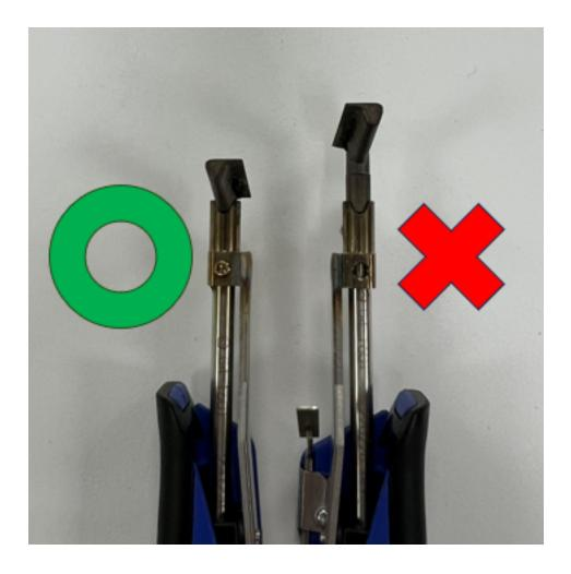
Dents in the blade caused by tightening the set screws when the blade is improperly inserted.
