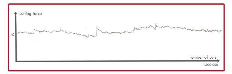
This cut test used 16 awg copper wire.
