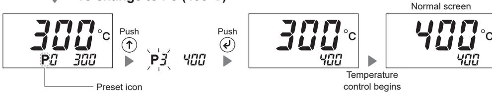
**NOTE** The registered temperature of each preset No. can be changed in "parameter No. 23." (See "8. Parameter settings")
