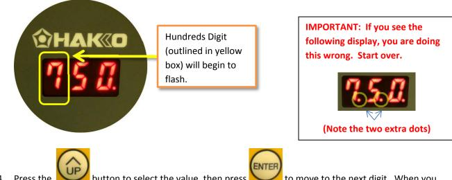
4. Press the button to select the value, then press button to move to the next digit. When you finish the last digit, the temperature is set.
