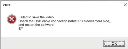
Is the USB cable loose or disconnected? (See "5-6. Connecting the USB cable")
