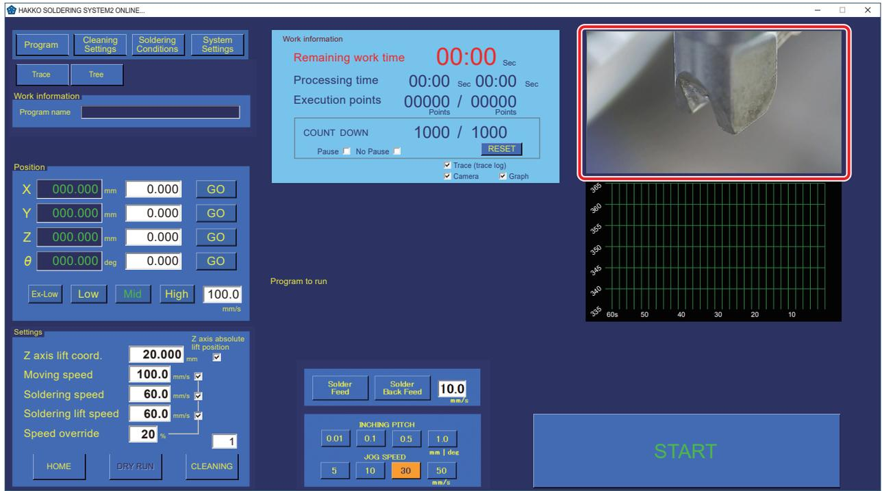
**3.** Adjust the arm/camera to the camera footage until the camera is in focus.
