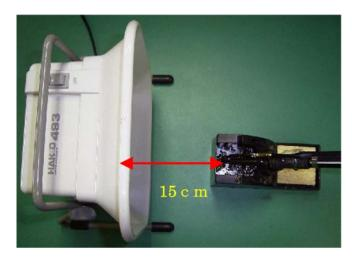
Set the handpiece on which the automatic solder feeder was mounted to the iron holder so that the distance between the smoke absorber and the tip end is 15cm.
