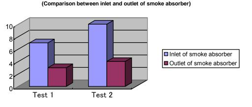
Test 1: Inlet of smoke absorber:  $7\mu g/m^3 \rightarrow$  Outlet of smoke absorber:  $3\mu g/m^3$ Test 2: Inlet of smoke absorber:  $10\mu g/m^3 \rightarrow$  Outlet of smoke absorber:  $4\mu g/m^3$
