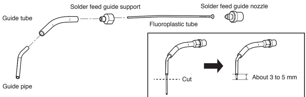
Turn the solder feed guide nozzle counterclockwise and remove the solder feed guide support. You can now install the fluoroplastic tube. Lastly, insert the guide pipe.
