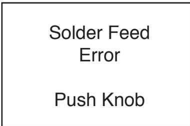
When the solder feed sensor detects "no solder" or "clogging", the HAKKO FU-500 will immediately stop the feed and show this error message on the LCD along with buzzer sound.
