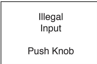
When an illegal input signal from the robot is detected, the HAKKO FU-500 will immediately stop the feed and show this error message on the LCD along with buzzer sound.
