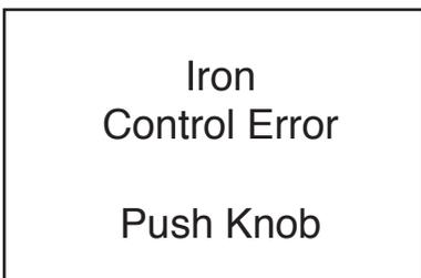
This error message is displayed when the HAKKO FU-601 ready input is "Not Ready" during Auto Mode or Manual Program Mode.
