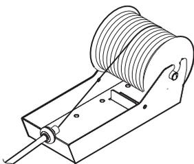
Ensure that solder is reeled out of the top of the bobbin.
