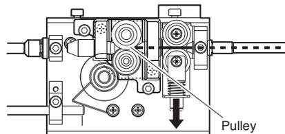
Draw solder through the tube unit and press the end of solder against the pulley of the solder feed pulley unit. With this condition, start the HAKKO FU-500 to feed solder until solder comes out of the end of the fluoroplastic tube.
