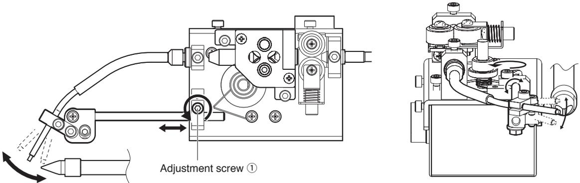
2. Loosening the adjustment screw ② will allow you to move the guide pipe as shown in the figure below. Move the guide pipe until solder comes into contact with the tip.
