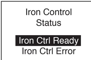
You can select which signal HAKKO FU-601 will output to the robot, Ready or Error.
