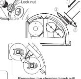
Removing the cleaning brush will make it easier to align the iron tip
