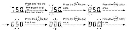
The desired temperature is saved to the system memory. Heater control will begin after the new set temperature is displayed.
