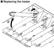
Measure the resistance of the heater. If the heater has ar open circuit, replace the heater
