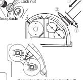
Removing the cleaning brush will make it easier to align the iron tip
