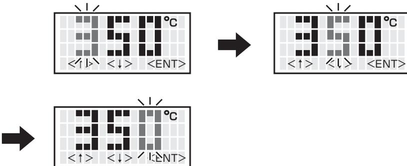
3. When desired figure is displayed, press the button to enter.
