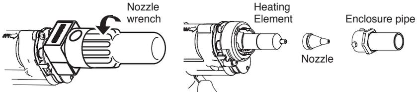
Remove the enclosure pipe and the nozzle with the attached wrench.
