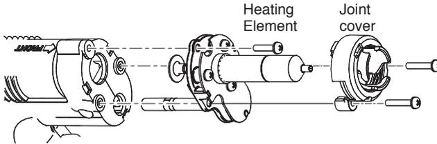
4. Replace the heating element. Assemble using the same procedure in reverse.
