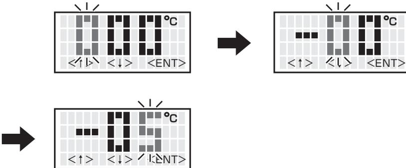
3. After entering the units digit, press the button to save the figure to the system memory and begin heater control with the new offset value.
