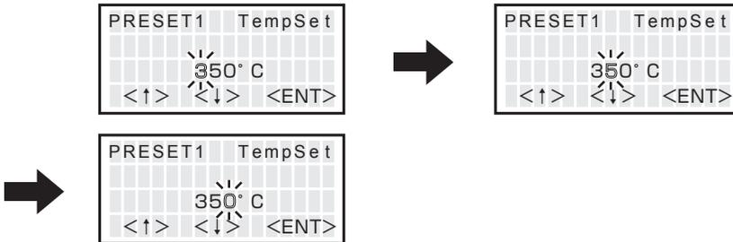
3. After entering the units digit, press the button to save the figure to the system memory and begin heater control with new setting temperature.
