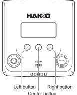
HAKKO FX-100 has 3 operation buttons. The operation executed by each button varies depending on what is on the display screen. The operation for each button is indicated at the bottom of the screen. Select the button according to the indication.
