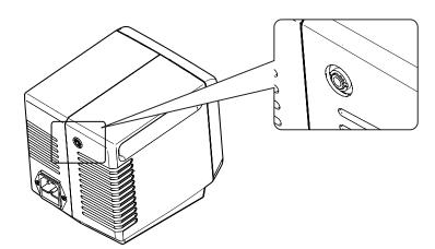
The port on the back of the station is used to display heater output on the external device. (not included)
